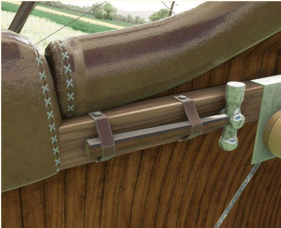
The “I’Hammer”: Used in case of a gun jam. Open the windshield, take the hammer, and bang bang bang. The hammer will work only if the windshield is down.
